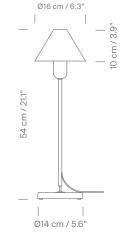
Brass, black anodized aluminium or natural anodized aluminium Chrome plated structure Cast zamak grey base 7,2W LED bulb included / 2.700°K
