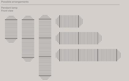
Pendant lighting system Washi Japanese paper shade Inner metallic structure Dimmable build-in LED / 2.700°K / CRI 95 Each circular module: L: 70W / M: 45W / S: 18W Each lineal module: 28W
